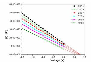
Fig. 3 – The reverse bias  $C^{-2}V$  characteristics of the Pd/V Schottky contact at different temperatures in the range 200-400 K
