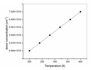
Fig. 4 – Temperature dependence of the donor concentration from experimental reverse bias  $C^{-2}$ -V characteristics of Pd/V Schottky contact
