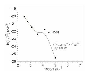
Fig. 6 – Richardson plot of  $\ln(I_0/T^2)$  versus  $10^3/T$  for Pd/V Schottky contact
