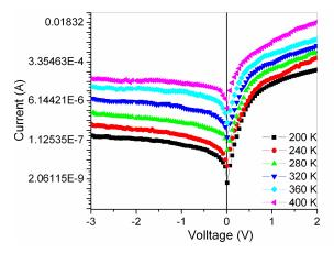
Fig. 1 – Typical forward and reverse current-voltage (I-V) characteristics of Pd/V Schottky contact on n-type InP in the temperature range of 200-400 K
