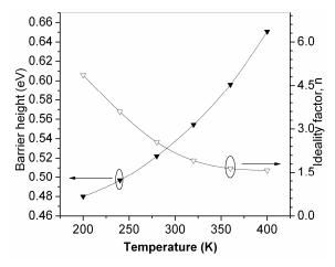
Fig. 2 – Temperature dependence plot of barrier height and ideality factor in range of 200-400 K
