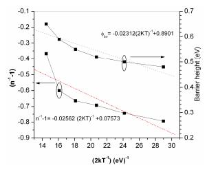
Fig. 5 – The zero-bias barrier height and ideality factor versus 1/2kT curves of the Pd/V Schottky contact according to Gaussian distribution of barrier heights
